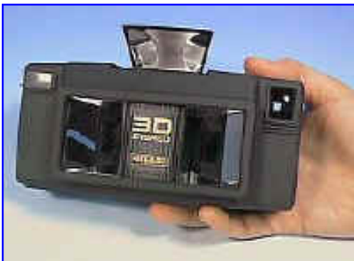
The Argus 3D Stereo Camera uses 35mm film. It has 2 matched 28mm lenses, 2 apertures (daylight and flash), and 1 shutter speed so everything is in focus from 2 1/2 feet to infinity. It also has a built-in pop-up flash. Image courtesy of Reel 3-D .
