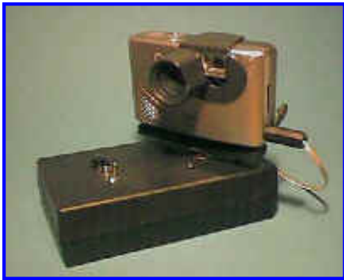
David Grenewetzki takes digital photos from rockets and remote control airplanes. To take panoramas with a remote control and a Kodak DC20 camera he designed and built this device that repeatedly turns the camera 45 degrees and takes a photo until eight pictures have been taken to cover a full 360 degrees. He uses a Tiffen wide-angle lens to increase the DC20's field-of-view so that I get full coverage with eight shots. He'll even sell you a kit to build your own. Courtesy of David Grenewetzki .
